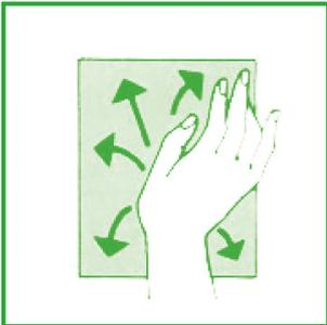
3. Use a hard rubber roller or a damp cloth to ensure airtight bond.
