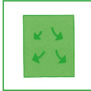
5. Remove any air bubbles and solution by pressure with a squeegee or rubber roller, beginning at the top edge.
